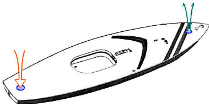
**Port Location Note:** It might be a good idea to Leak Test the hull prior to installing any inspection ports. In the event repairs will require an inspection port in a non-typical location this would help to avoid adding more ports than absolutely necessary. Ventilating can be just as successful through ports located almost anywhere so repair needs would take precedent.
