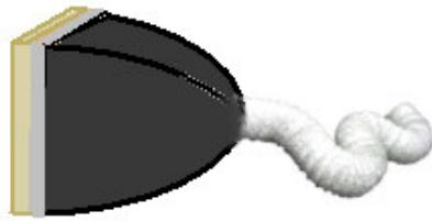
With a single port, fan-forced air can be piped in using a shop-vac hose or a small dryer vent hose so long as the hose size leaves enough room through the inspection port for exhaust air to exit around it. A dual port, fan forced system gives the best outside air exchange.
